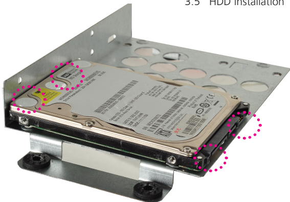
3.5" HDD installation (screw slots are on the bottom of the tray)
